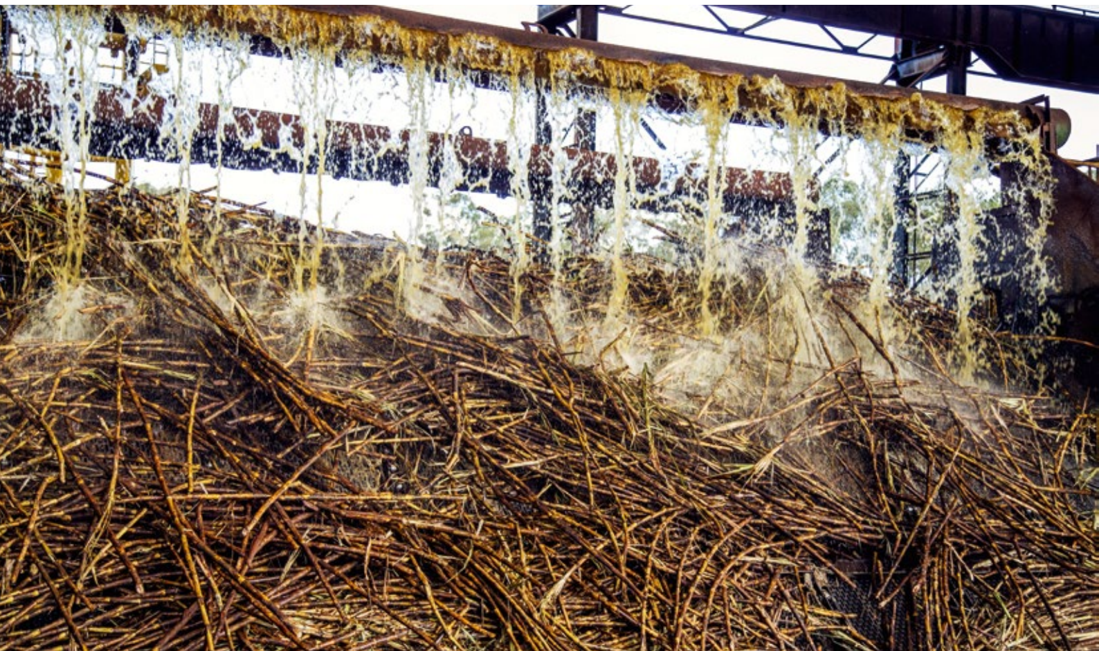
Figure 4.1: Washing of sugarcane stalks in a bioethanol manufacturing plant.
